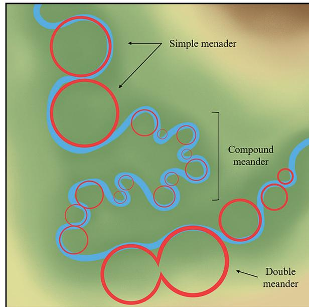
Fig. 5. Determining the type of the meander.
