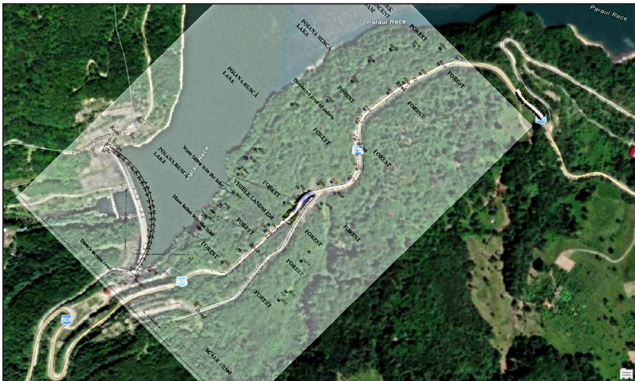
**Fig. 3.** Overview from ArcGIS representing the overlapping of the topo-geodetic network plan with the airborne photogrammetry surveys.
