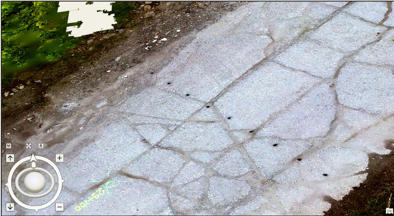
**Fig. 10.** The quality of the orthophotomosaic allows for detecting the end of the GPR profiles marked with spray on the pavement.
