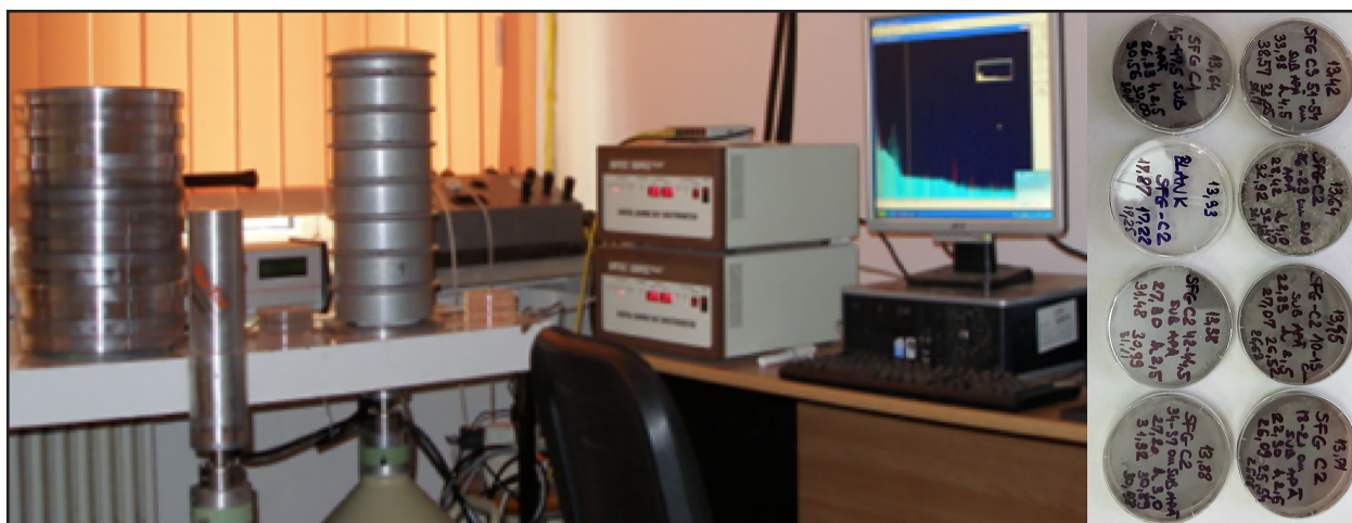
Fig. 4. HPGe detectors and related electronics; Petri dishes with sediment samples
