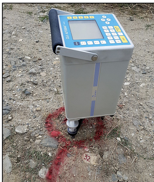
Fig. 4. The equipment used for gravimetric measurements CG5 Autograv Scintrex
