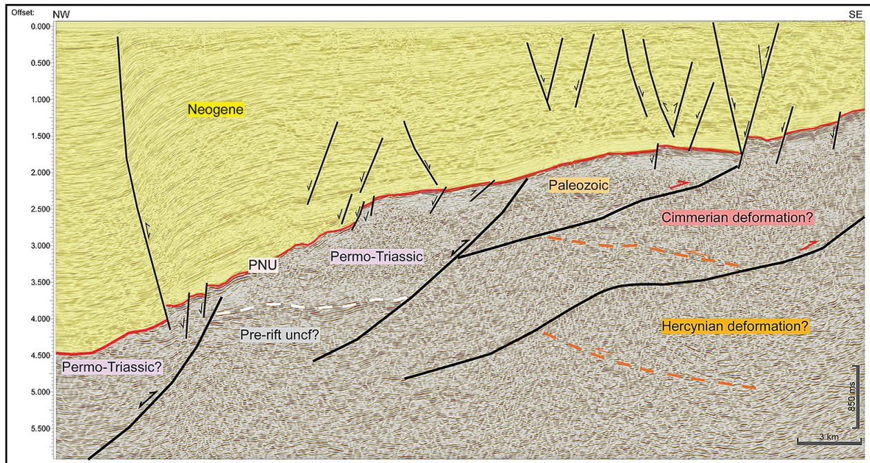
**Fig. 7.** 2D seismic line acquired and processed in 2012 by OMVP and Hunt Oil, illustrating the poor-quality seismic character visible below the PNU, and a possible interpretation based on Nord Dobrogea Orogen outcrops observations.
