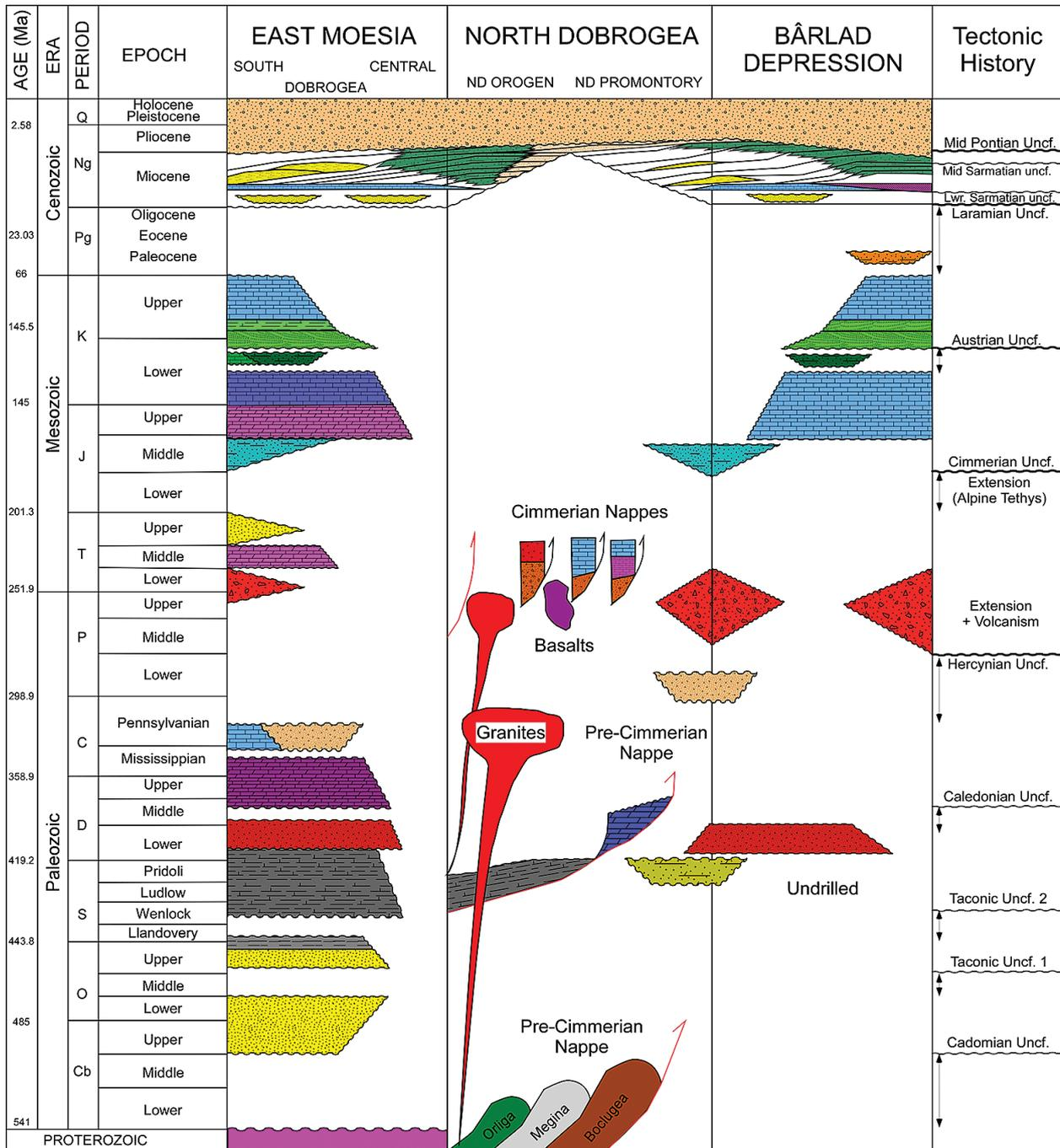
**Fig. 3.** Chronostratigraphic chart illustrating the differences and similarities among the three juxtaposed basins (East Moesia, North Dobrogea Orogen and Bârlad Depression), (Săndulescu, 1984, Vinogradov *et al.*, 1997, Mutihac *et al.*, 2004, Seghedi, 2012). Chronostratigraphic scale after IGR Lithofacial Atlas; Unconf.: unconformity.
