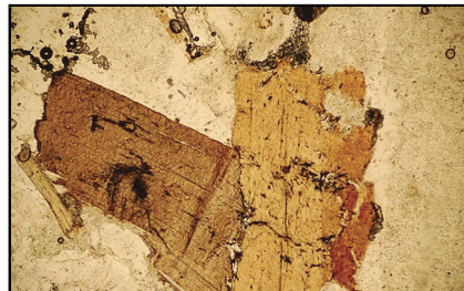
Mineralogy: Red Bi with halo around the Zr inclu- sions, metamictic effect- Qz-Plg .
