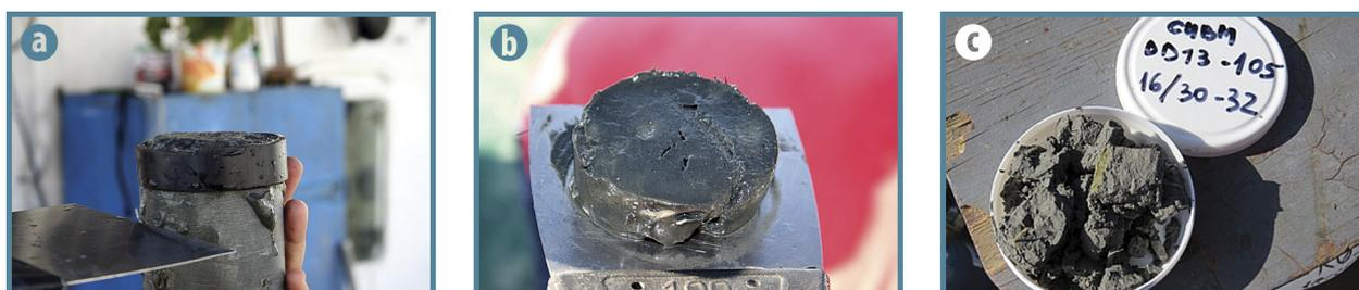
Fig. 3. Slicing the sediment core at adequate levels (a), the resulted sediment slice (sample) (b), and a sample within a box (station code, slice number and depth interval are written on its cover), prepared to be send to a lab for analyses (c).
