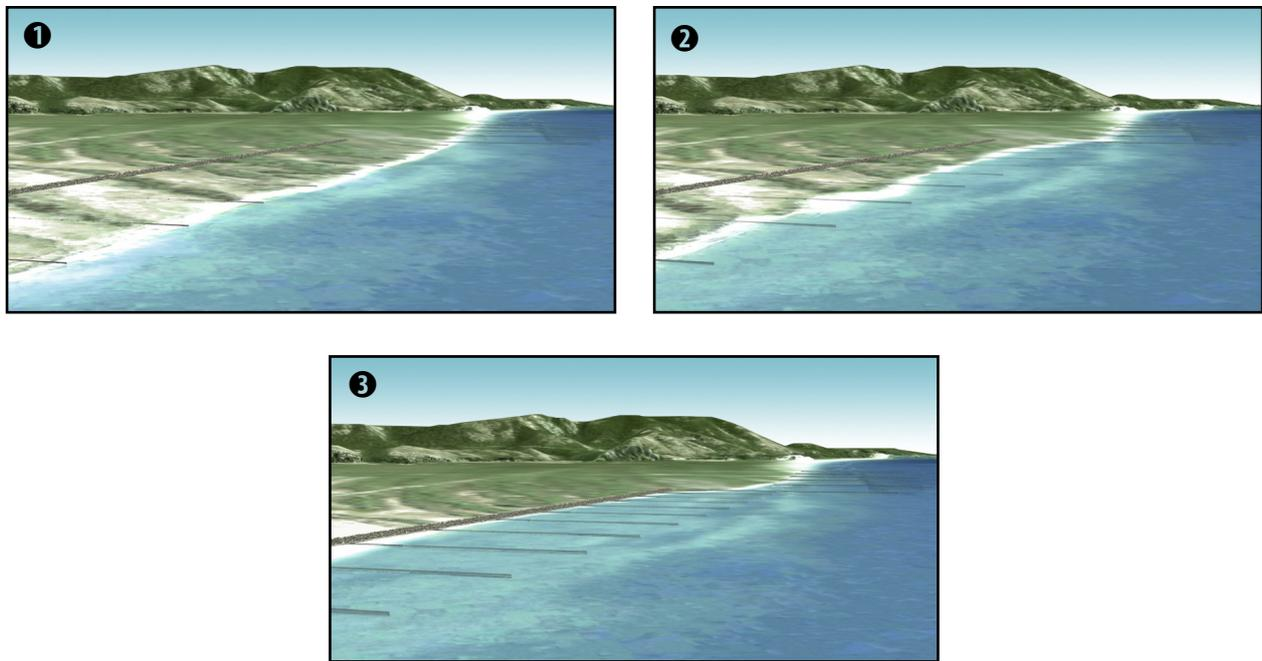
**Fig. 12** Managed realignment project along the southern side of Ombrone river delta (Rendering: Nevio Danelon, DST-UNIFI). **Legend:** 1) Retreated seawall and buried groins. 2) Partial exhumation of groins, which start acting as submerged structures 3) Utmost position of the shoreline with the seawall able to protect inland areas from extreme storms.
