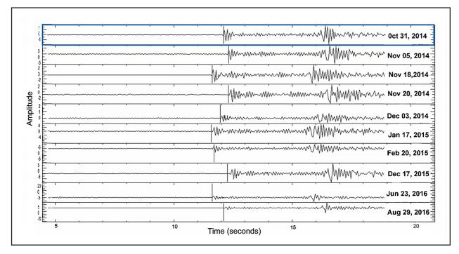
**Fig. 5.** Waveform display for the template of 31/10/2014 – 23:11:18 (first trace, highlighted in blue) and associated waveforms that correlate with CC factor above 0.9 recorded at HERR (Herculane) station displayed with SAC software. A Butterworth bandpass filter of 1-5 Hz is applied.
