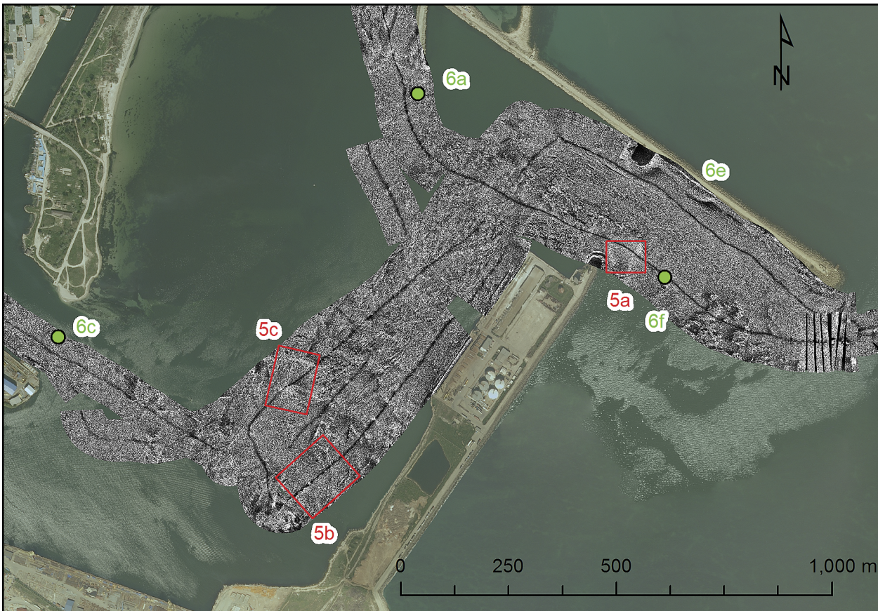
Fig. 3. Mosaicked sonograms comprising the central Mangalia harbour area and the entrance from the Black Sea. The position of mosaic cropped details and analysed objects presented in the following figures (Fig. 5, 6 and 8) is pinpointed by numbers, borders and arrows.
