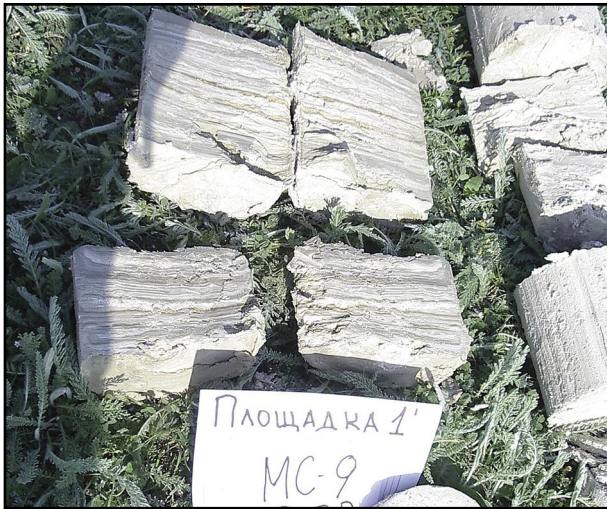
Pl. II, Fig. 1. Drill-core of aragonite clay: The fine horizontal lamination is clearly seen.
