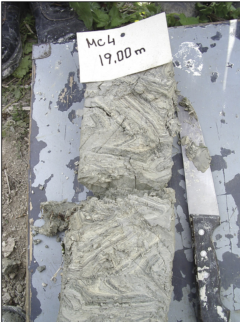
Pl. II, Fig. 1. Drill-core of aragonite clay: The fine horizontal lamination is clearly seen.
