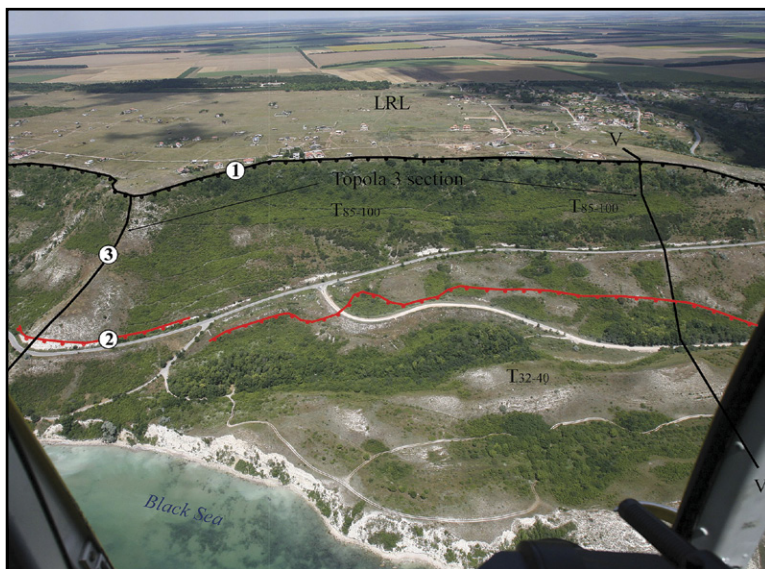
Pl. I, Fig. 2. View of the Topola 3 section: LRL – Lower Romanian Level; 1 – high scarp of a provisionally stabilized two-storey landslide; 2 – low landslide scarp of an active landslide; 3 – flanks of the landslide; V-V – profile line; T 85-100 – terrace at an absolute elevation, m.
