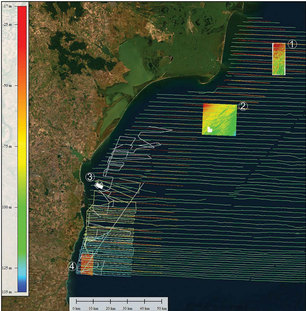
**Fig. 4.** Existing data in the area of interest (1, 2, 4 panels of DTM, 3 panel of DTM, SSS, and SBP): green lines – SBP 3.5 kHz; orange lines – MBES; yellow – MBES+SBP (chirp 2-12 kHz); cyan – MBES + SBP (chirp 2-12 kHz); white – MBES+SBP (chirp 2-12 kHz).
