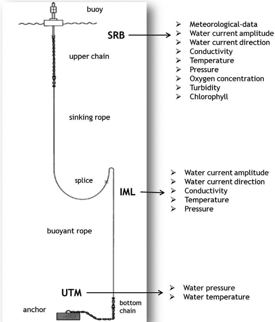
**Fig. 6.** Types of data collected from the EUXINUS buoys. Abbreviations: SRB, surface relay buoy; IML, intermediate module layer; UTM, underwater tsunamometer module.
