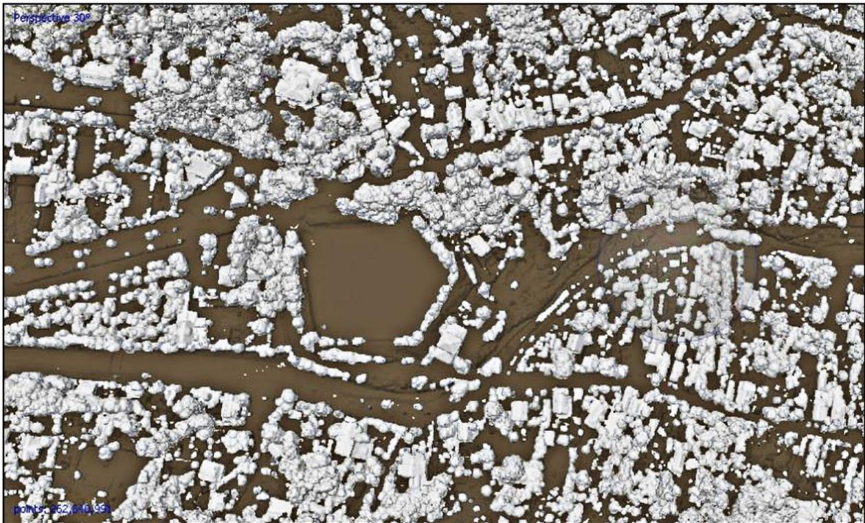
**Fig. 3.** The classified point cloud, in which the white areas represent the remaining unclassified points (vegetation and buildings).
