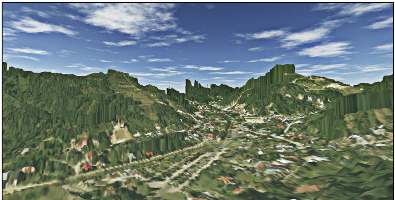
**Fig. 8.** A 3D perspective of the Digital Elevation Model (with an orthoimage mapped to the vertices) showing the variation in elevation.
